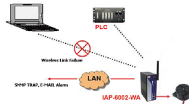
Link Monitor and Alarm
